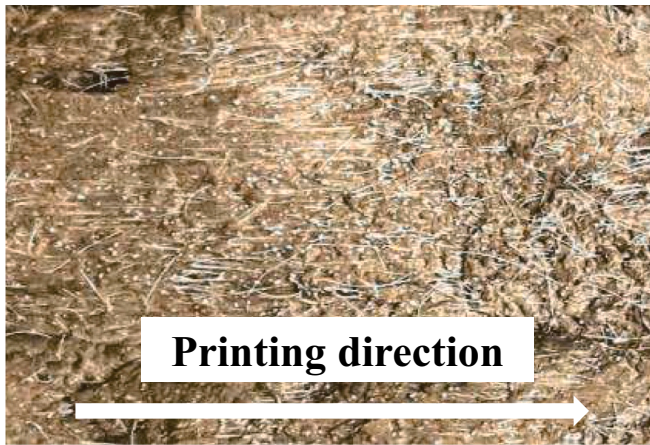
Fig. 11. Fiber alignment observed in 3DP-ECC.
