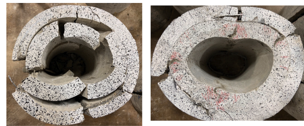
(a) Mortar-repaired pipe (b) ECC-repaired pipe
