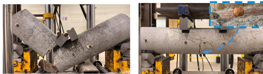
(a) Mortar-repaired pipe
