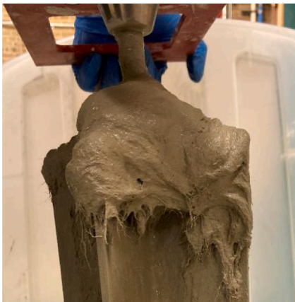
(c) Fiber clog at 60 min.
