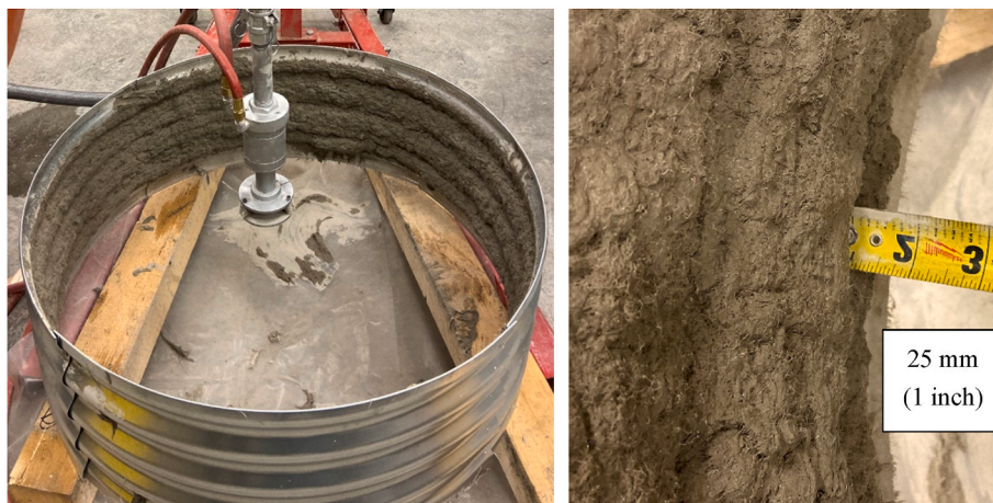
Fig. 16. Centrifugal sprayed ECC on a 900 mm-diameter corrugated metal pipe.
