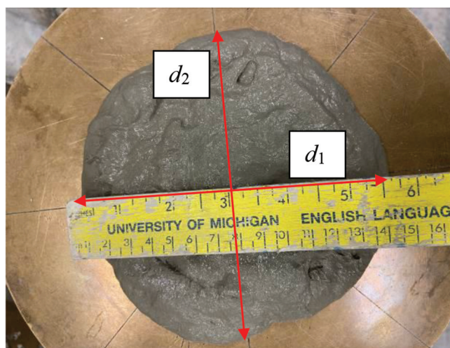
Fig. 2—Flow table test of fresh ECC.
