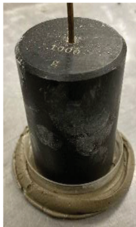
(a) Bulge-deformation of LC3-M with 1 kg weight at 20 min.
