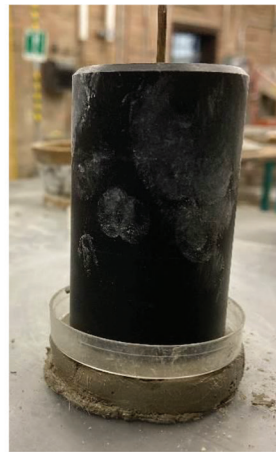
(b) LC3-ECC retained 80% of the original height with 1 kg weight at 20 min.
