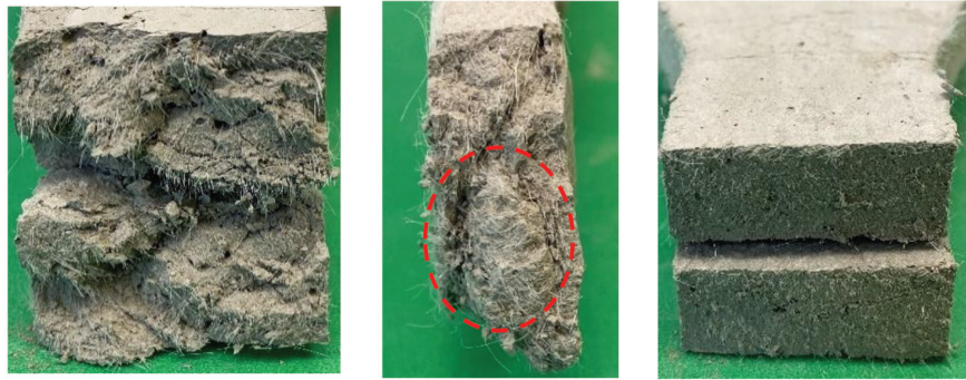
(d) Fracture surface with minor balling of fiber. (e) Fiber clump. (f) Fracture surface of nozzle-cast-LC3 ECC with limited fibers.
