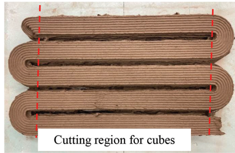
(a) 3DP LC3-ECC for compressive and split tensile tests (Printed with six layers of filaments by 50 mm width, 600 mm length, and 10 mm thickness).
