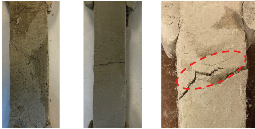
(a) Saturated cracks. (b) Unsaturated cracks (c) Local failure due to the print flow
