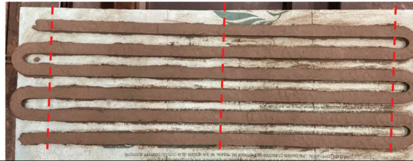
(b) 3DP LC3-ECC for the direct tensile test (Printed with one layer of the filament by 30 mm width, 800 mm length, and 13 mm thickness).
