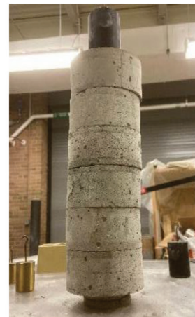
(c) LC3-ECC retained 80% of the original height with 7 kg weight at 80 min.
