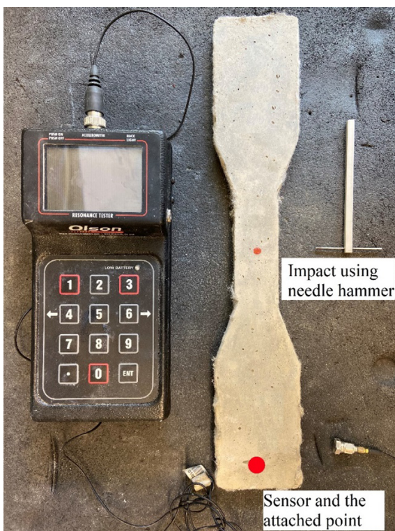
Fig. 4. Resonance frequency test set-up.
