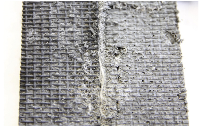
Fig. 5. Opposing faces exposed after layer debonding and sectioning of a VCP-mesh specimen. Interlayer mineral bridges or pillars are formed through the mesh apertures and subsequently severed during loading, leaving a marked surface roughness that may contribute a desired resistance to layer sliding. Interfaces in the PP-mesh scheme have a similar appearance, but with larger mesh apertures and thus larger interlayer mineral pillars.
