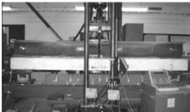
Fig. 7—Laboratory test setup and instrumentation of specimen. (Dimensions shown in mm.)
