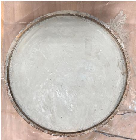
Fig. 3. Expansion steel ring test, with three strain gauges attached on the external surface separated by 120° of the steel ring.
