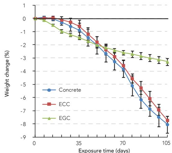
Figure 2: Weight change of cement concrete, ECC, and EGC in the sulfuric acid exposure test.
