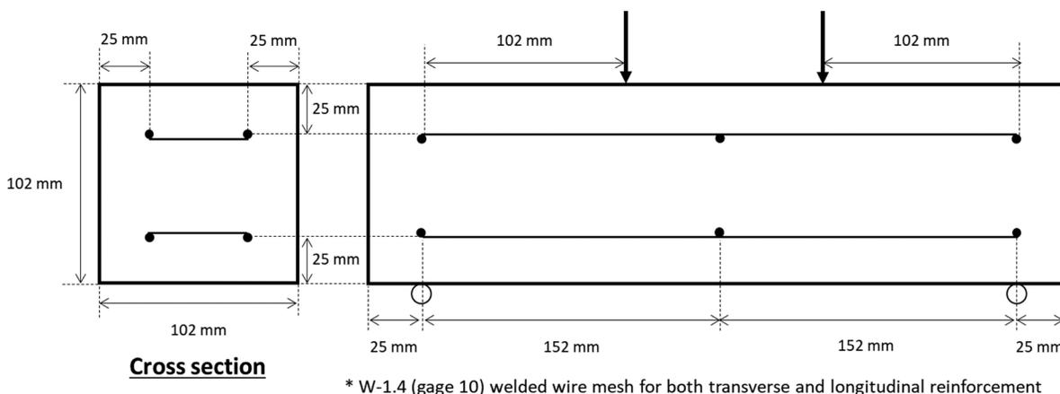
Figure 1: RC beam design and testing setup of four-point bending.
