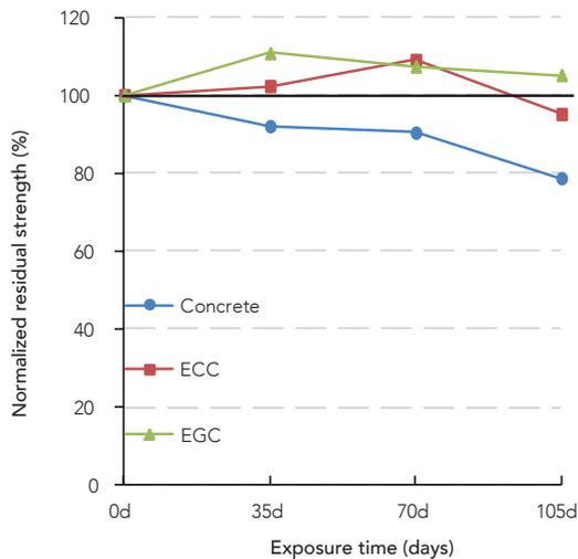
Figure 3: Normalized residual strength of cement concrete, ECC and EGC.
