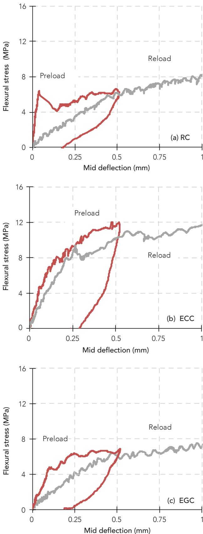
Figure 4: Typical bending curves of RC, ECC, and EGC in preloading and reloading. For easy comparison of bending stiffness, the curves are plotted up to a mid-deflection of 1 mm.
