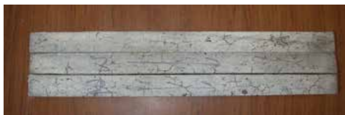
Fig. 4: Typical formation of map cracking due to ASR damage in mortars without PVA fibers after 30 days of high alkaline exposure
