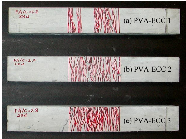
Fig. 12 Beam bottom surface shown increasingly saturated microcracks after bending test for PVA-ECC 1-3 (Microcracks are magnified with thick pen for the constant moment span length only).
