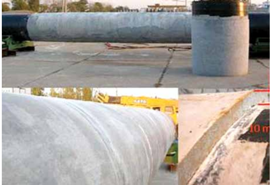
Figure 5. ECC surface coating for oil/gas pipe protection. Image courtesy of Lepech et al, 2010.
