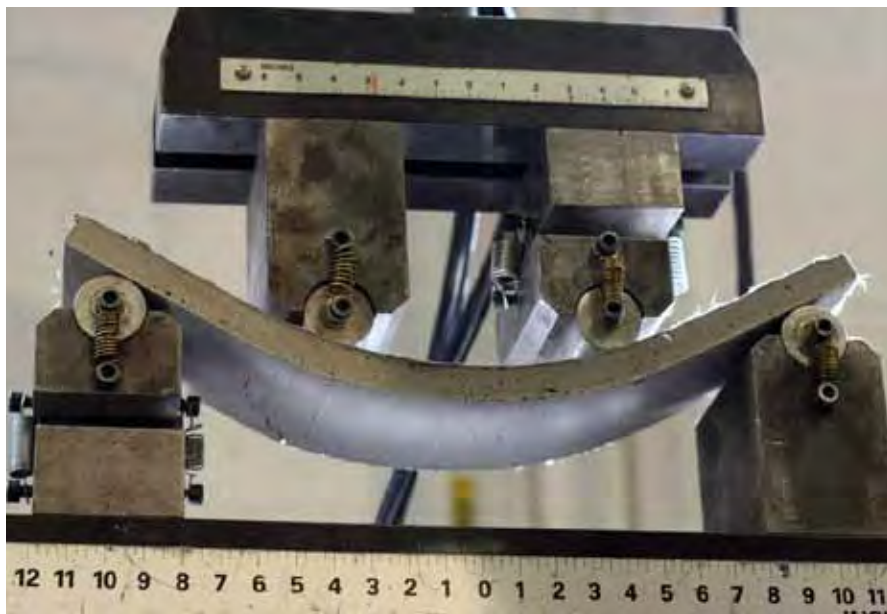
Figure 3. This image shows the extreme flexing capabilities of ECC under a large bending load. Image courtesy of UM News Services.
