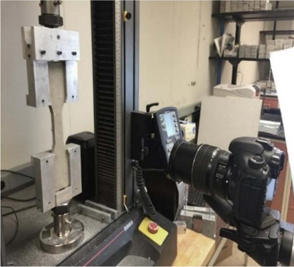
Fig. 3. Tensile test setup with camera capturing pictures.
