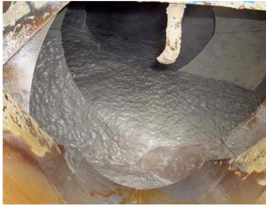
FIGURE 24.7: Creamy texture appearance of fresh ECC in mixing drum of a ready-mix truck (Lepech and Li, 2007).
