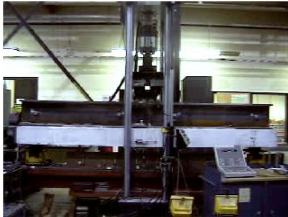
FIGURE 24.14: Flexural fatigue testing of ECC link-slab element (Kim et al, 2004).
