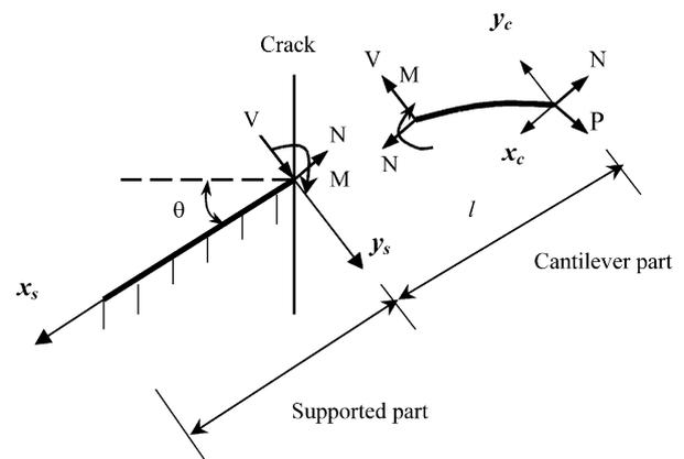
Fig. 2. Loads of supported and cantilevered parts of fiber as pulled.
