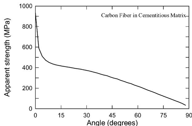
Fig. 3. Effect of inclination angle on carbon fiber apparent strength.
