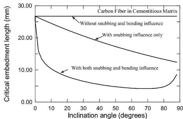
Fig. 4. Influence of inclination angle on carbon fiber critical embedment length.
