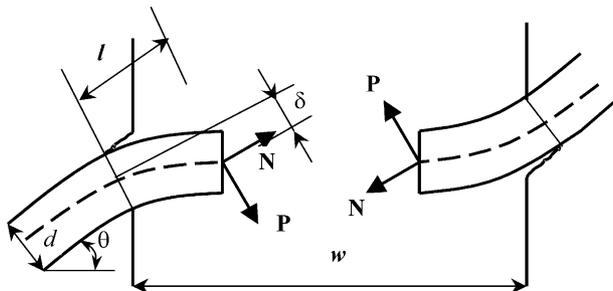
Fig. 1. Bending of fiber across crack.
