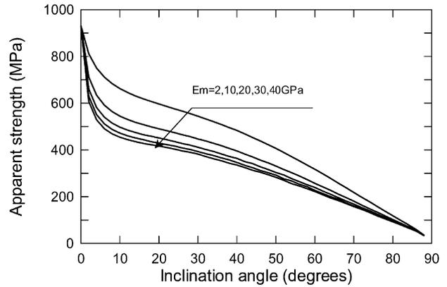
Fig. 5. Effect of matrix elastic modulus on fiber apparent strength.
