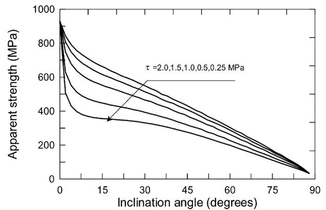
Fig. 7. Effect of fiber/matrix bond strength on fiber apparent strength.
