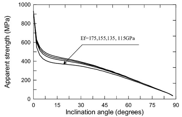
Fig. 6. Effect of fiber elastic modulus on fiber apparent strength.
