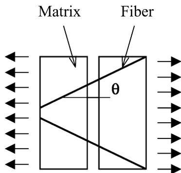
Fig. 8. Test setup for fiber rupture.
