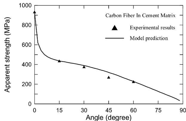
Fig. 9. Comparison between model prediction and experimental results on fiber apparent strength.
