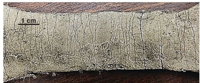
FIGURE 4 Crack pattern of ECC under tension.
