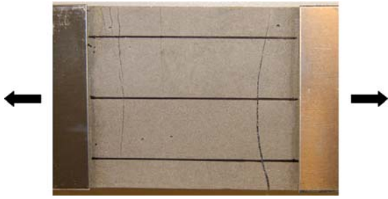
Fig. 7 Illustration of the measurement of loaded crack width
