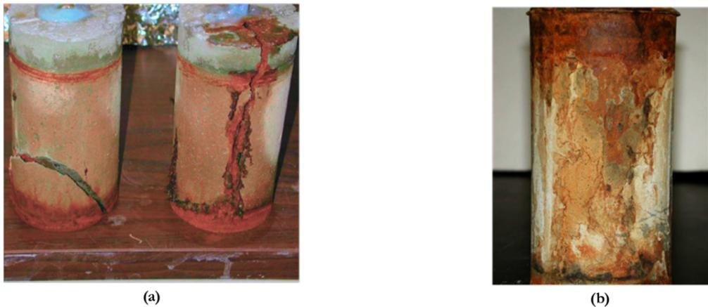
**Figure 5** (a) Spalled mortar specimen after 95 hours accelerated corrosion, and (b) ECC specimen after 350 hours accelerated corrosion.
