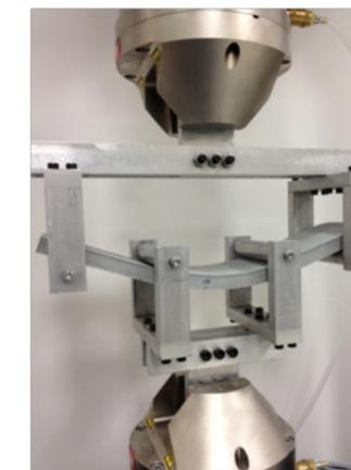
**Figure 2** ECC flexes without brittle fracture
