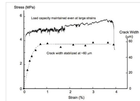
**Figure 1** ECC has tensile ductility several hundred times that of normal concrete, and crack width self-controlled to less than 100  $\mu\text{m}$ .
