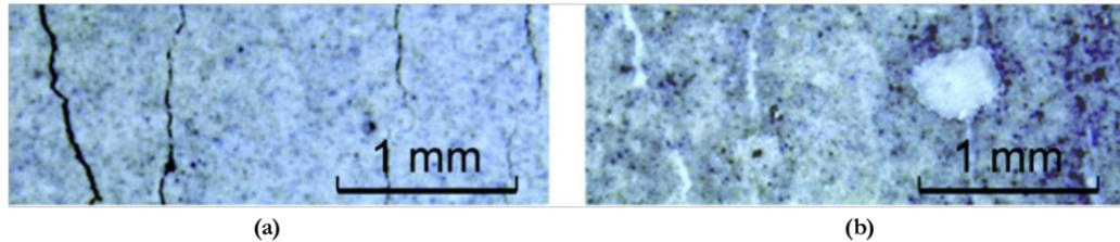
**Figure 4** ECC self-heals crack damage when exposed to water and air. (a) Before and (b) after healing
