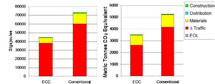
**Figure 8** Life cycle (a) primary energy consumption and (b) CO<sub>2</sub> equivalent for the ECC shows about 40% less than that of conventional bridge deck systems.
