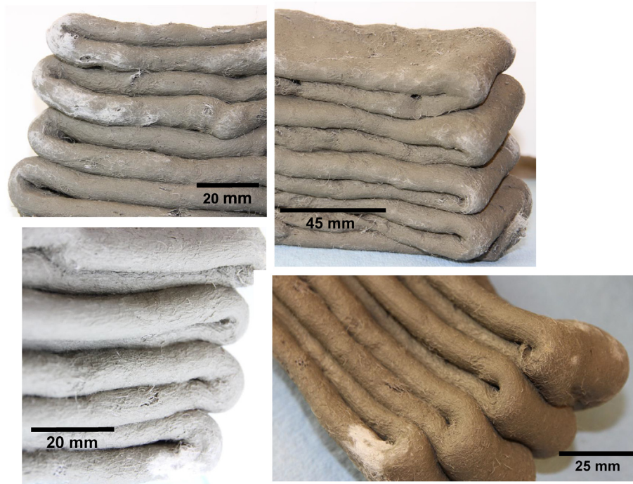
Fig. 23. Large-scale printing approximations produced with the Mix 5 composition, showing a combination of extrudability, buildability and appropriate hardening/early strength behavior.
