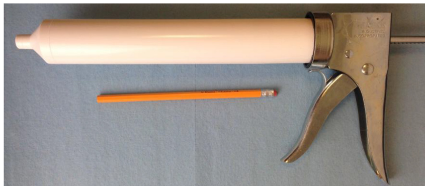
Fig. 4. A mechanically actuated, manually operated caulk-gun apparatus, shown with a pencil for scale, was used as a means of extrusion for a small-scale approximation of the final step of the 3D printing process. Nozzle diameters 8–13 mm were used.
