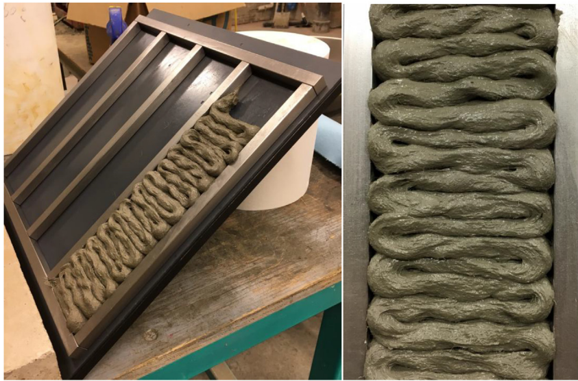
Fig. 16. Preparation of the print pattern to be used in interlayer bonding testing of Mix 4 via the approximated 3D printing technique. Coupon shaped specimens were sectioned from the print pattern and tested in tension with the loading axis normal to the bond lines between filaments.
