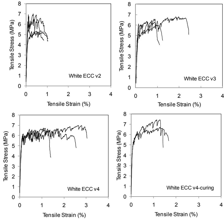
Figure 5: Uniaxial tensile stress-strain curves of white ECC v2 to v4
