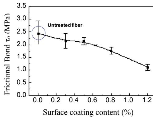
Figure 4: Fiber/matrix interface frictional bond as a function of surface coating content [5]
