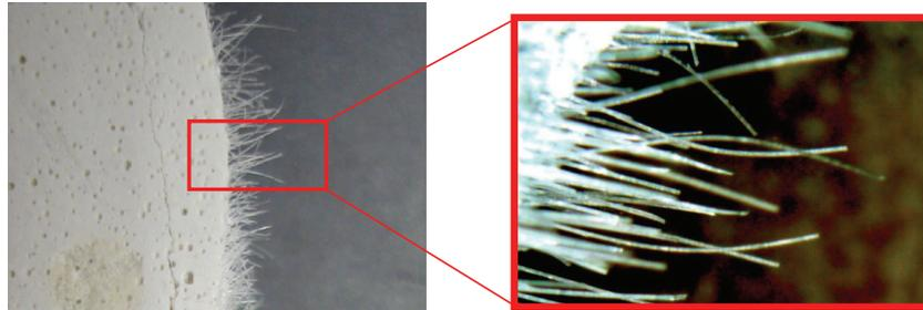
Figure 3: Microscopic observation of fracture surface of white ECC v1
