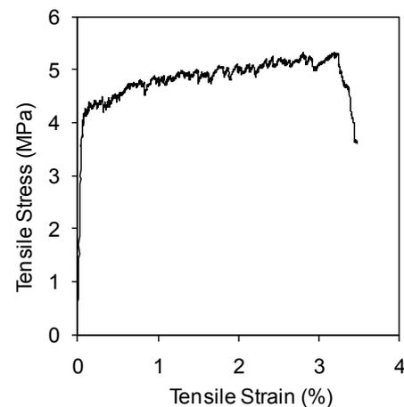
Figure 1: A typical uniaxial tensile stress-strain curve of standard PVA-ECC M45
