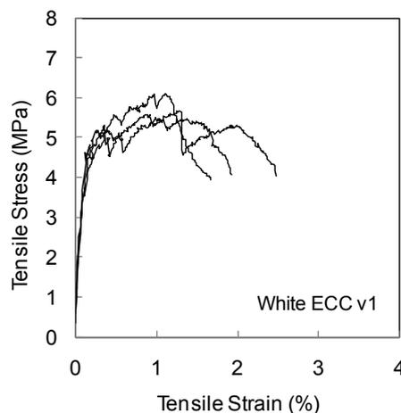
Figure 2: Uniaxial tensile stress-strain curves of white ECC v1
